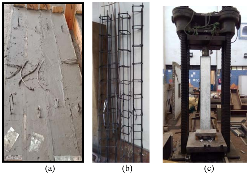
Fig.2: Experimental stages, a) Casting Columns; b) RFT. Basalt & Steel Cages c) Test Setup.
